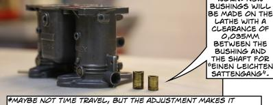
\*MAYBE NOT TIME TRAVEL, BUT THE ADJUSTMENT MAKES IT POSSIBLE TO ACHIEVE 100% AIR FLOW SYNCHRONICITY BETWEEN THE TWO THROTTLE BORES.
