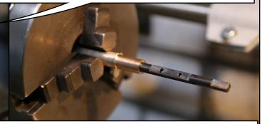
THE BUSHINGS ARE GLUED IN THE PIVOT POINTS USING LOCTITE GO3. DURING THIS STEP THE SHAFTS ARE FITTED TO ENSURE CORRECT ALIGNMENT.
