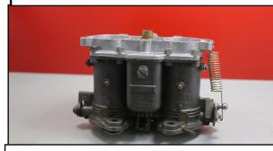
THE SPLIT SHAFT SOLEX USED ON THE LATER 912'S (G9') HAD AN ADJUSTMENT BLOCK IN BETWEEN TWO SEPARATE THROTTLE SHAFTS TO BE ABLE TO ADJUST THE BUTTERFLIES INDIVIDUALLY. THIS IS WHAT MAKES TIME TRAVEL POSSIBLE.\*
