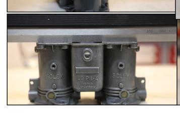
LEAKAGE DOES NOT OCCUR. THE PREVIOUS MECHANIC HAD ALREADY INSTALLED BRONZE BUSHINGS IN THE PIVOT POINTS. SADLY THESE WERE ALSO WORN. NEW
