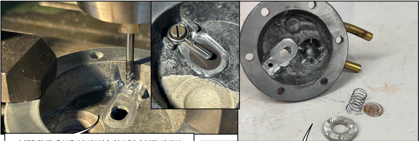
CORRODED PUMP HOUSINGS CAN BE SAVED IF THE PITTING IS NOT TOO DEEP. A VERY SMALL END MILL CAN BE USED TO REWORK THE SEALING SURFACE.
