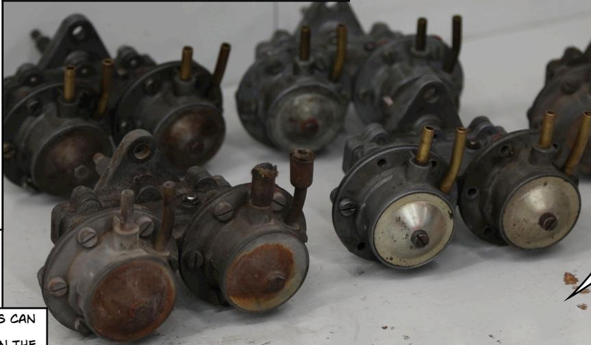
OVERHAULING A FUEL PUMP WHICH HAS BEEN USED ALL OF ITS LIFE IS USUALLY EASIER THAN ONE THAT HAS SAT FOR A LONG TIME. WITH TIME THE ZAMAK WILL START TO CORRODE. A BIT OF CLEANING AND A FEW NEW GASKETS WON'T CUT IT.
