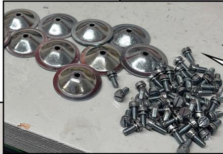
ALL HARDWARE IS ZINC PLATED. YOU CAN BUY NEW SCREWS BUT THE SCREW HEADS WON'T BE THE CORRECT SHAPE. DETAILS, DETAILS, DETAILS!
