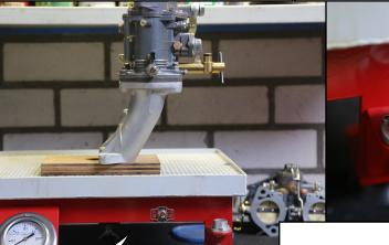
DAS WERKZEUG ZUR SCHWIMMERGEHÄUSE-KRAFTSTOFFNIVEAUPRÜFUNG UND EINSPRITZMENGE-EINSTELLUNG. IN SHORT A LEVEL TABLE WITH AN ELECTRICAL FUEL PUMP AND A RESERVOIR TO CATCH THE SPILLED FUEL. FOR THE ADJUSTMENT OF THE FLOAT LEVEL IT IS IMPORTANT FOR THE CARBURETTOR TO BE LEVEL. THIS WILL PREVENT A WRONG READING OF THE FUEL LEVEL IN THE FLOAT BOWL.
