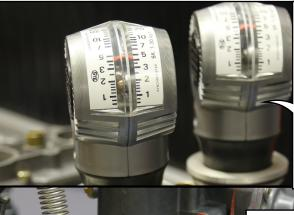
WITH AIR FLOW METERS THE AMOUNT OF AIR FLOWING THROUGH THE BORES CAN BE MEASURED IN KG/H. THE AIR FLOW ON ALL FOUR BORES IS ADJUSTED TO READ 3,5-4 KG/H. THIS WILL ALLOW FOR THE ENGINE TO RUN IDLE AT \$50-900 RPM.
